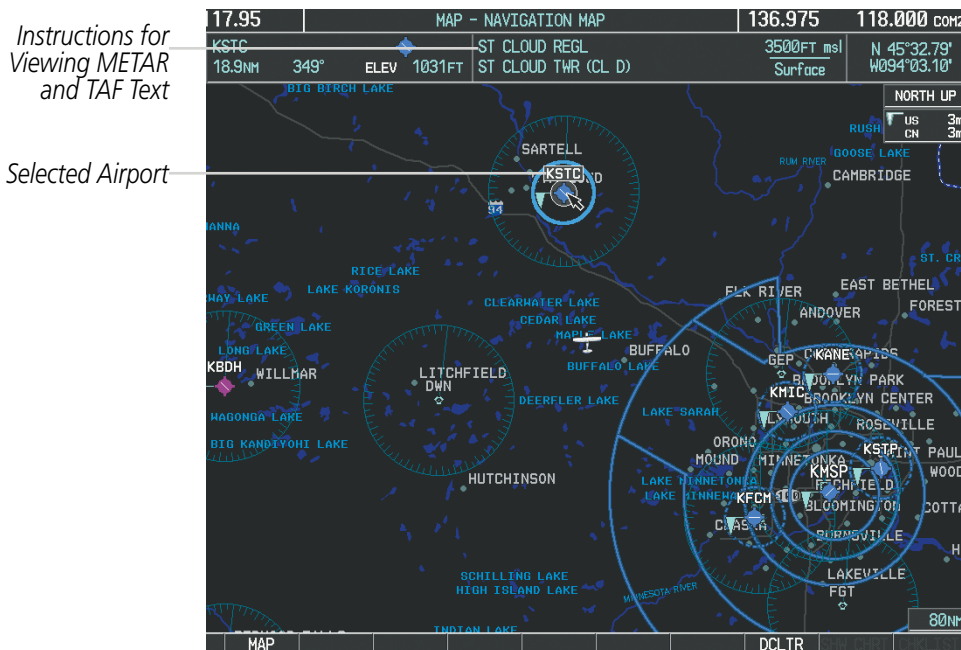
Figure 6-78 METAR Flags on the Weather Data Link Page
