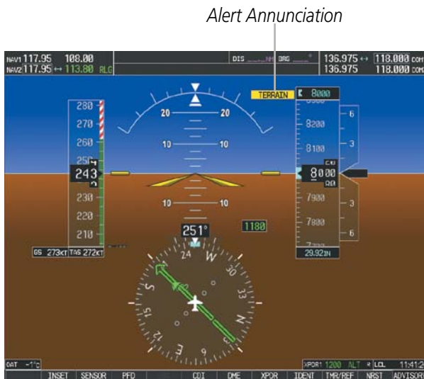
Figure 6-143 TAWS-B PFD Alert Annunciation
