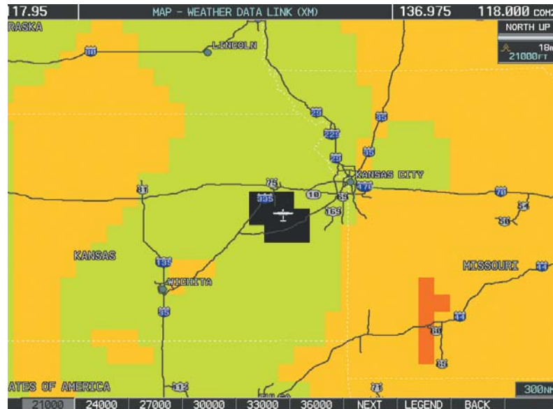
Figure 6-44 Turbulence Data at 21,000 Feet
