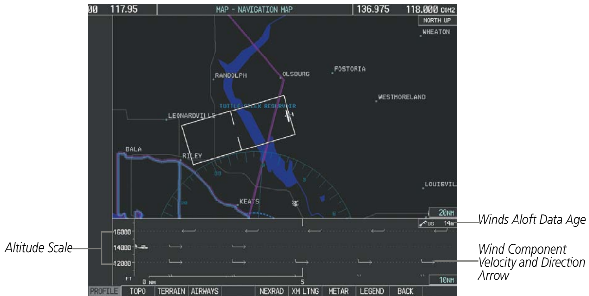
Figure 6-34 Navigation Map Page with Winds Aloft Data on Profile View
