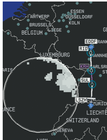
Figure 6-67 GFDS Weather Data Request Results with Precipitation and Infrared Satellite Displayed
