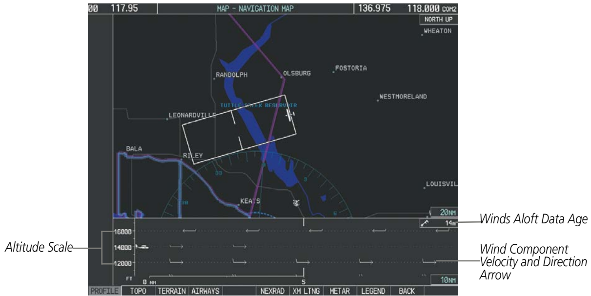
Figure 6-83 Navigation Map Page with Winds Aloft Data on Profile View
