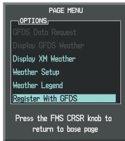
Figure 6-55 Select Register With GFDS
