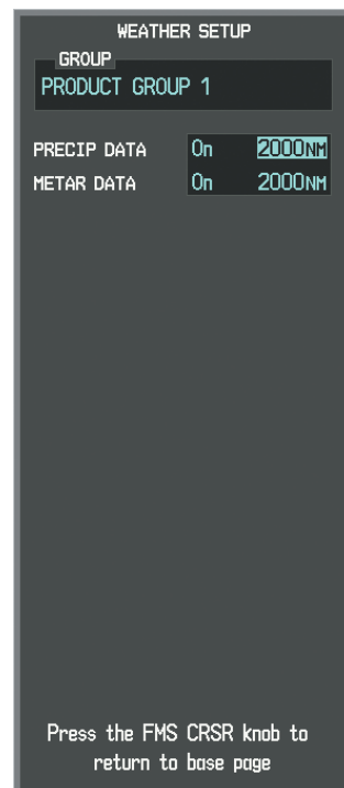
Figure 6-101 Weather Data Link Page Setup Menu
