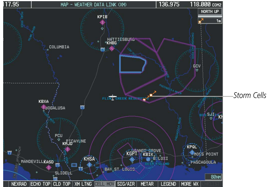
Figure 6-20 Cell Movement Data
